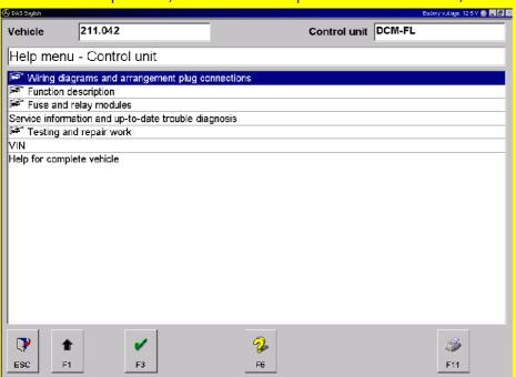
If you press F6 a second time while in the Help menu for model series and control units, the "Changes and new features" and "DAS operating tips" help menus are displayed. This "Help on Help" is only available for passenger cars.
