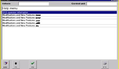
After a model series is selected, the Help function then relates to aspects of the currently selected vehicle, such as wiring diagrams, connector pin assignments, functional descriptions and abbreviations.
